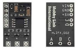
Points A thru E are the control and lighting pins for the board. VIN and GND are your connections for power. The board is tolerant for both 9V and 12V DC, so you can use either one to power the board. +5V is a 5V output pin, but it is not used for the Planes circuit, so you can leave it disconnected. You can solder wire directly to these thru-hole connections, use male header pins, or any other method you prefer.
