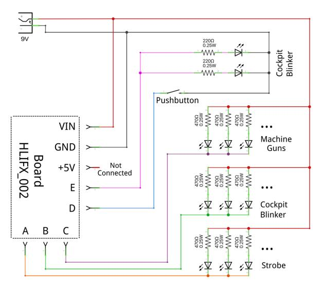
The strobing LEDs, machine gun LEDs and one set of cockpit LEDs will be driven from your 9V-12V power supply, so, if you choose to wire them yourself:
