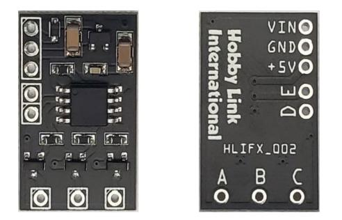
Points **A** thru **E** are the control and lighting pins for the board. **VIN** and **GND** are your connections for power. **The board is tolerant for both 9V and 12V DC**, so that you can use either one to power the board. +5V is a 5V output pin, **but it is not used for the Batwing circuit**, so you can leave it disconnected. You can solder a wire directly to these thru-hole connections, use male header pins, or any other method you prefer.
